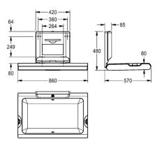
CAMBRINO horizontal baby changing table for wall mounting, made of polypropylene with antibacterial Biocote® protection, white colour, hinged, with integrated shock absorber for safe opening and closing, nylon safety belt and hooks on both sides, lockable dispenser for single-use paper covers in Interfold folding with maximum width 260 mm. Certified according to EN 12221-1 and EN 12221-2. Including mounting material and 80 single-use paper covers.
